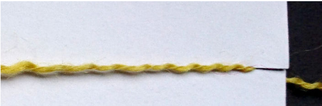
Figure 145: To prepare a yarn for scanning, cut a notch at each side of a paperboard, and anchor a thread in the notches.
