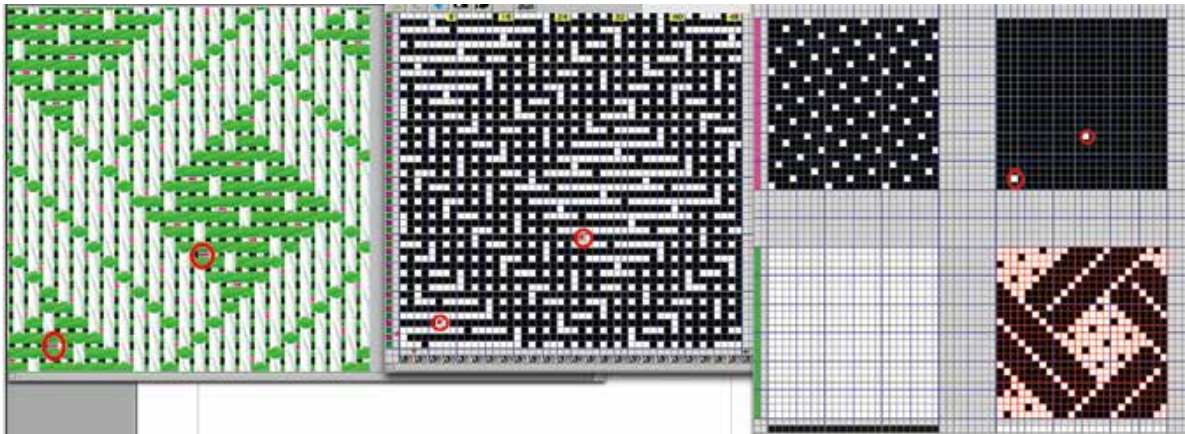
Figure 10. Lattice with hidden stitchers circled in red
